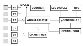
POLY PHASE ENERGY METER USING THE ADSST-EM-2030
