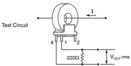
The CS60 Series measures current from 5 to 100 amps rms. Applications include sensing branch circuit overload and detecting load drop or shutdown. The sensor functions as the encapsulated secondary of a current transformer, while the conductor carrying the current to be measured serves as the "one turn primary." Sensitivity may be enhanced by increasing primary turns.
