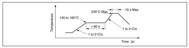
Figure 1 An Example of Infrared Rays Reflow Conditions
