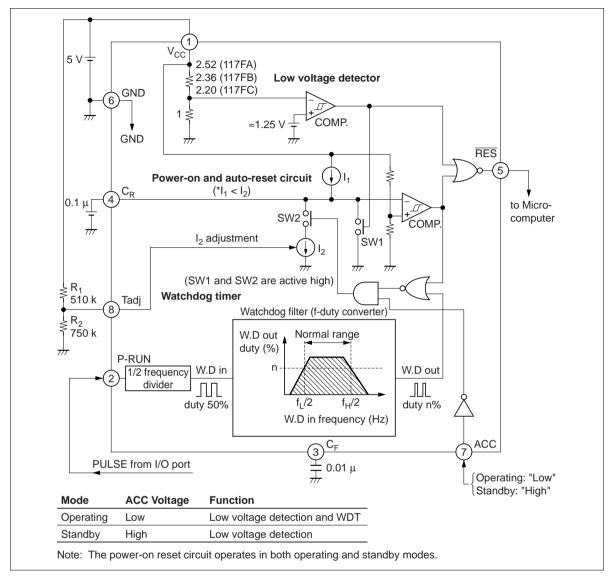
The HA16117F consists of a low voltage detector, power-on and auto-reset circuit, and watchdog timer.
