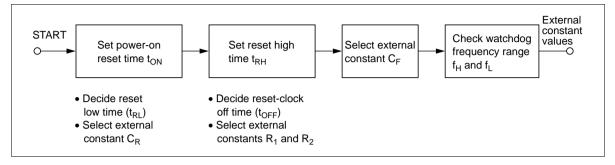
Figure 4 Procedure for Selecting External Constants
