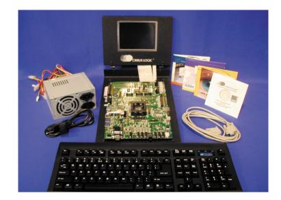
The EDB9312 development kit is a convenient, user-friendly, systemoriented platform that provides design engineers with the ability to evaluate and utilize the EP9312 processor capabilities, features, and state-of-the-art technology. By fully leveraging an impressive selection of integrated peripherals in a complete system environment, designers can develop a multitude of next-generation consumer and industrial electronic products from a single platform design.
