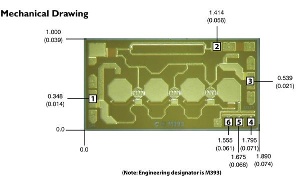
Units: millimeters (inches) Bond pad dimensions are shown to center of bond pad. Thickness: 0.076 + -0.010 (0.003 + -0.0004), Backside is ground, Bond Pad/Backside Metallization: Gold All DC Bond Pads are  $0.080 \times 0.080 (0.003 \times 0.003)$ . All RF Bond Pads are  $0.180 \times 0.080 (0.007 \times 0.003)$ . Bond pad centers are approximately 0.109 (0.004) from the edge of the chip. Dicing tolerance: +/-0.005 (+/-0.0002). Approximate weight: 1.172 mg
