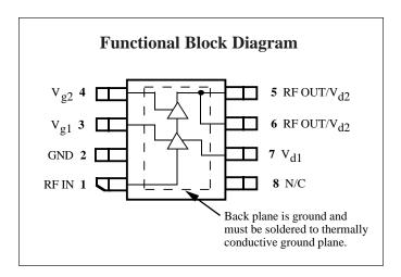
mum performance and flexibility. The CMM0336 is packaged in a low-cost, space efficient SO-8 power package that gives excellent electrical stability and thermal handling performance with a  $R_{\Theta}$  of less than 18° C/W. The part is designed to require minimal external circuitry for bias matching, simplifying design and keeping board space and cost to a minimum.
