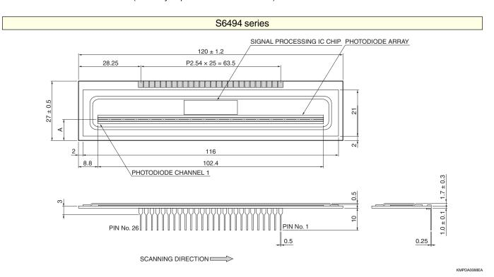
A: Distance from the bottom of the board to the center of the active area  $86494-64:9.35\pm0.2$ ,  $86494-128:9.05\pm0.2$
