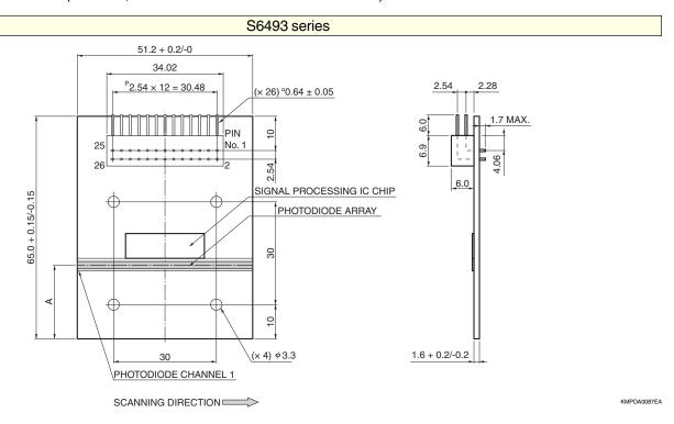
A: Distance from the bottom of the board to the center of the active area  $6493-64:21.15\pm0.2$ ,  $6493-128:21.35\pm0.2$  Board: G10 glass epoxy
