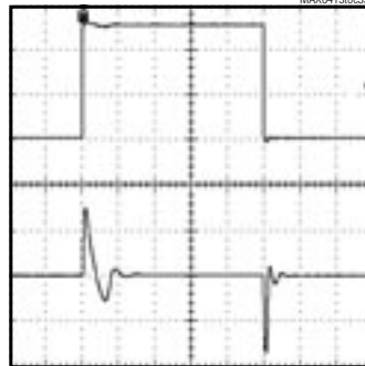
LOAD TRANSIENT ( V_{OUT} = 2.5V , C_{OUT} = 1\mu F , 0 TO -2mA)
