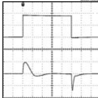
LOAD TRANSIENT ( V_{OUT} = 10V , C_{OUT} = 1\mu F , 0 TO 20mA)
