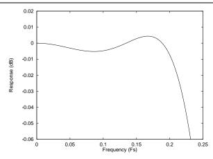
Figure 45 ADC Digital Filter Frequency Response –Type 2
