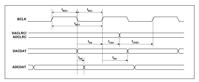
Figure 6 Digital Audio Data Timing – Slave Mode
