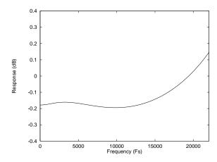
Figure 51 De-Emphasis Frequency Response (44.1kHz)
