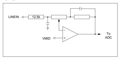
Figure 9 Line Input Schematic
