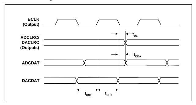
Figure 4 Digital Audio Data Timing – Master Mode
