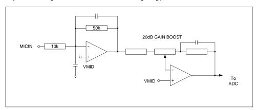
Figure 11 Microphone Input Schematic
