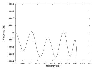
Figure 33 DAC Digital Filter Frequency Response -Type 0
