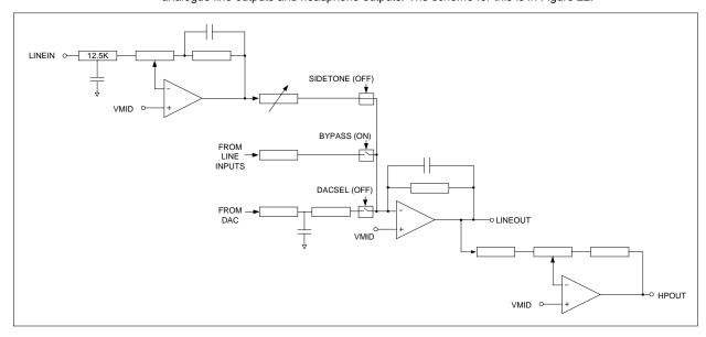
Figure 22 Signal Routing in Bypass Mode
