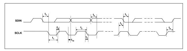
Figure 8 Program Register Input Timing – 2-Wire MPU Serial Control Mode
