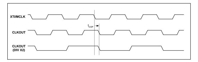
Figure 2 Clock Out Timing Requirements
