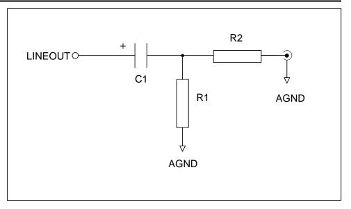
Figure 19 Line Outputs Application Drawing
