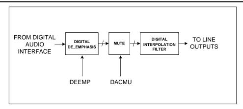
Figure 16 DAC Filter Schematic
