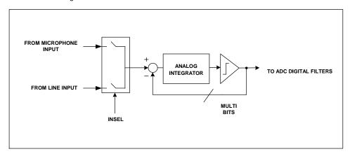
Figure 14 Multi-Bit Oversampling Sigma Delta ADC Schematic
