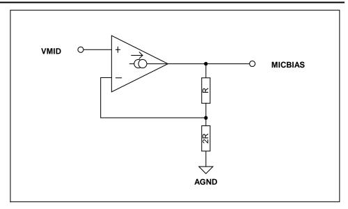
Figure 13 Microphone Bias Schematic
