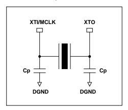
Figure 24 Crystal Oscillator Application Circuit
