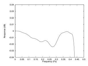
Figure 35 DAC Digital Filter Frequency Response -Type 1
