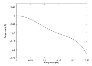
Figure 39 DAC Digital Filter Frequency Response -Type 3
