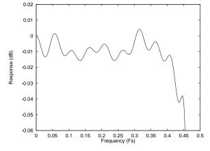
Figure 43 ADC Digital Filter Frequency Response –Type 1
