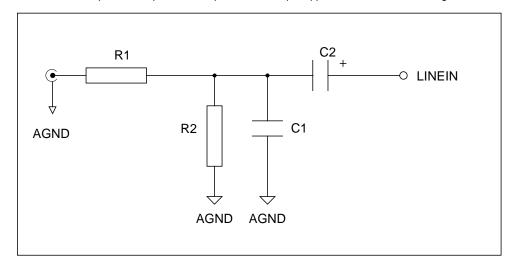
Figure 10 Line Input Application Drawing
