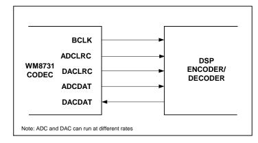
Figure 3 Master Mode Connection
