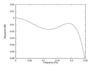
Figure 47 ADC Digital Filter Frequency Response –Type 3
