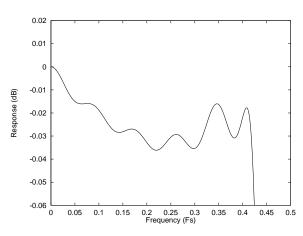
Figure 41 ADC Digital Filter Frequency Response -Type 0
