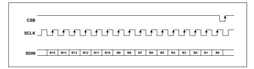
Figure 31 3-Wire Serial Interface
