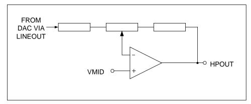
Figure 20 Headphone Amplifier Schematic
