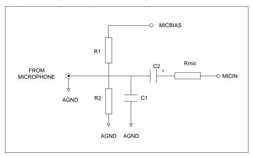
Figure 12 Microphone Input and Bias Application Drawing
