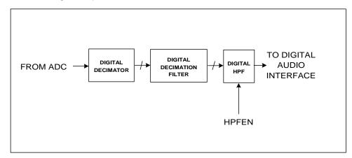
Figure 15 ADC Digital Filter
