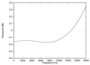
Figure 49 De-Emphasis Frequency Response (32kHz)
