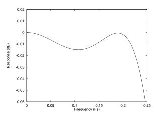
Figure 37 DAC Digital Filter Frequency Response -Type 2
