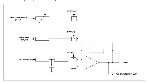
Figure 18 Line Output Schematic
