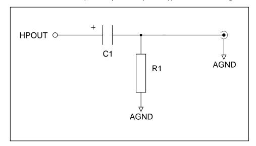
Figure 21 Headphone Output Application Drawing
