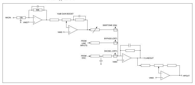
Figure 23 Side Tone Mode Schematic
