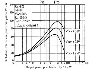
The total device power dissipation when hybrid IC's  $V_{CC} = \pm 28V$  and  $R_L = 6\Omega$ , for a continuous sine wave signal, is a maximum of 81W, as is in Pd-P<sub>O</sub> graph.
