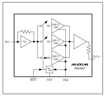
Figure 3. Functional Diagram
