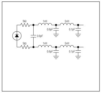
Figure 2. Photodiode and Header Model
