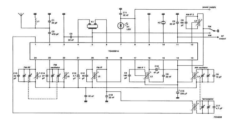
Fig.5 Application circuit.
