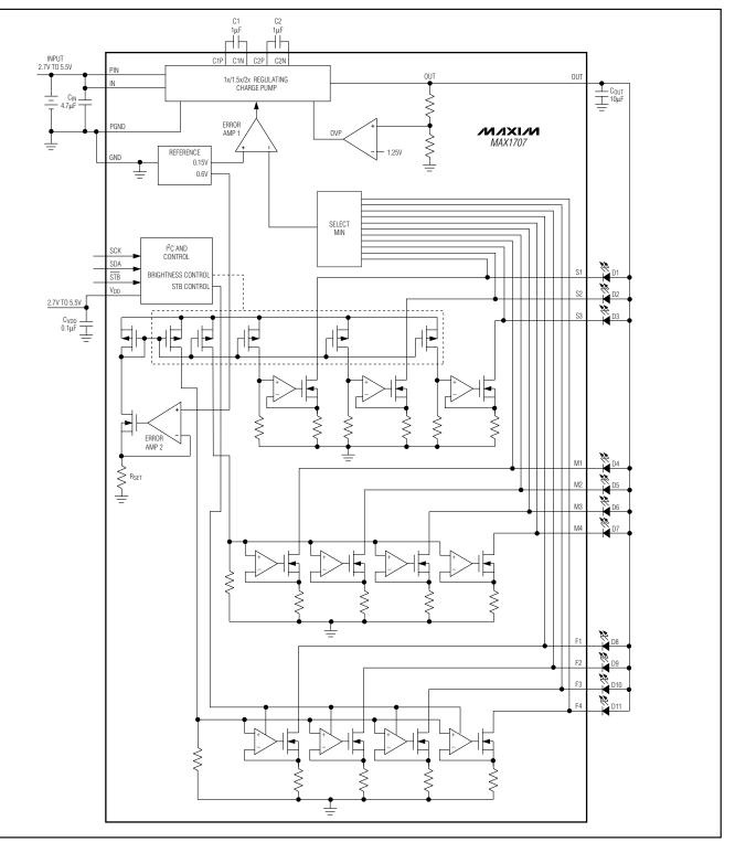
Figure 1. Functional Diagram
