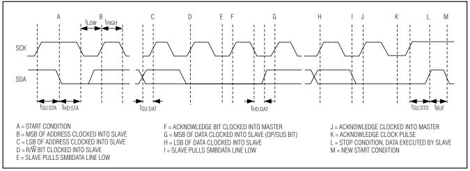
Figure 2. I<sup>2</sup>C Timing Diagram
