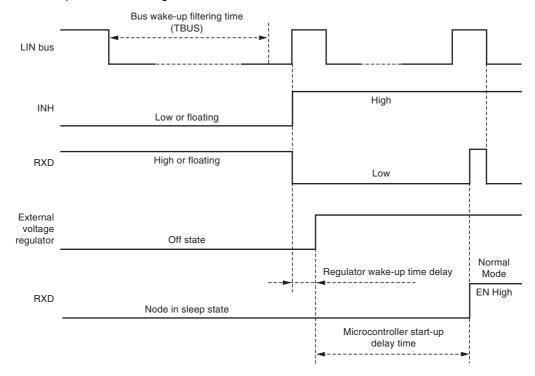
Figure 3-3. Wake-up from Wake-up Switch
