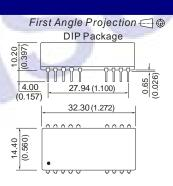
RECOMMENDED FOOTPRINT Top view,grid:2.54mm(0.1inch) diameter:1.00mm(0.039inch)
