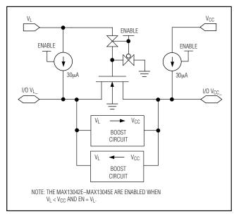
Figure 4. Simplified Functional Diagram for One I/O Line
