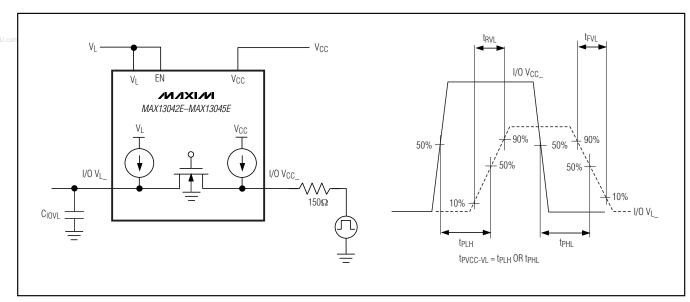
Figure 2. Push-Pull Driving I/O V<sub>CC</sub>\_ Test Circuit and Timing
