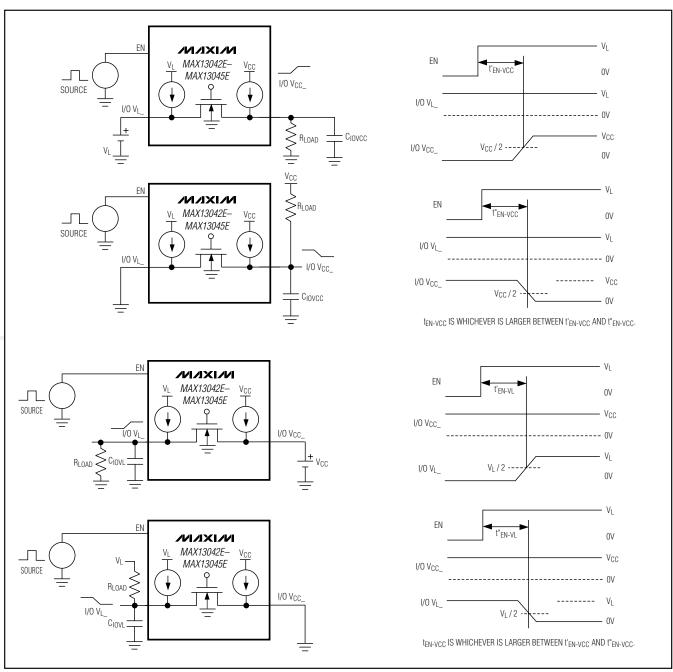
Figure 3. Enable Test Circuit and Timing
