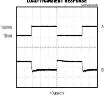
A: LOAD CURRENT B: OUTPUT VOLTAGE: AC-COUPLED, 100mV/div
