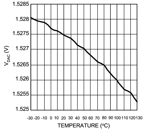
V DAC vs Temperature External Ref, DAC Trim @ 1.525V
