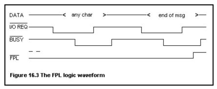
Notice that the FPL signal is removed at the end of the message, while the CY545B is still Busy, but after the I/O Request has been driven high again.
