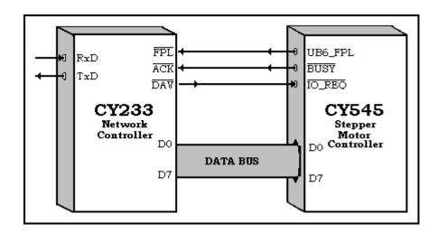
The CY233 Network Control chip allows you to connect up to 255 devices to a single RS-232 serial communications line such as an IBM-PC COM1 or COM2 port, with unique addresses assigned to each device. The CY233 Network is ideal for distributed systems where central control is required but very high speed communication is unnecessary.
