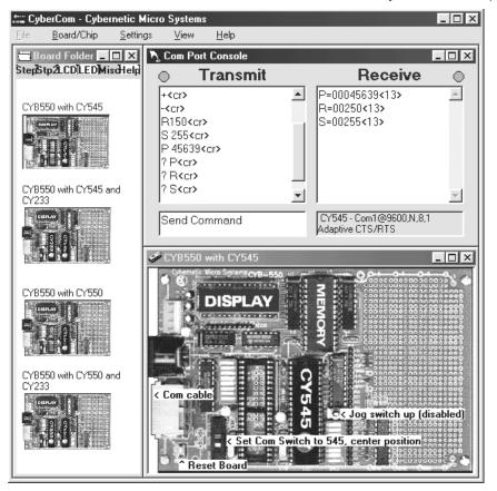
data-length, parity, stopbits, and CTS/RTS. Typing is buffered at the keyboard until the Enter key sends the entire string to the serial port. A Carriage return terminator is optional.
