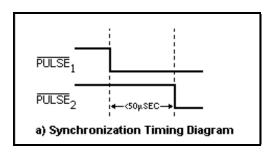
Two CY545s, executing similar programs from external memory, may be synchronized as shown in the figures. The master CY545 can control a USERBIT line of the slave CY545 via the Bit command, to set or clear a user bit. The slave CY545 is started first, with an Execute command, and executes a Wait command and waits until the USERBIT line is driven low by the Bit command executed by the master CY545, when it receives the (second) Execute command. Both CY545s then proceed
