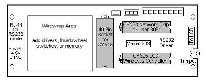
The board contains a socket that will accept the CY545, and allows it to communicate serially with the CY325. Also included are an RS-232 interface and RJ-11 jacks for serial connection to the board. A wire wrap area makes it possible to add the motor driver interface, the local external memory, and thumbwheel switch interface for the CY545.
