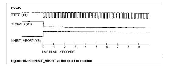
Once the motor is moving, the INHIBIT\_ABORT signal may be used to slow down and stop a motion before the CY545 reaches the target position. Using the signal in this way provides a controlled early stop to the motion.
