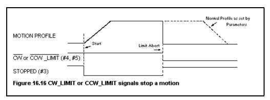
Also, if a limit signal is low at the beginning of a motion, the motion will not be taken. The CY545 immediately aborts the motion without taking any steps. Normal motions are allowed in the opposite direction. Example waveforms are shown above.
