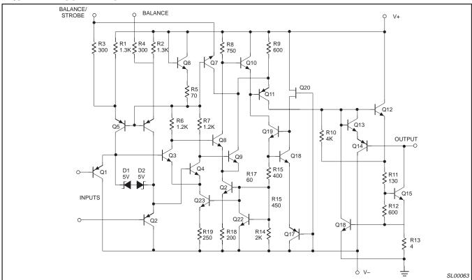
Figure 2. Equivalent Schematic
