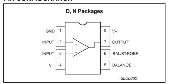
Figure 1. Pin Configuration
