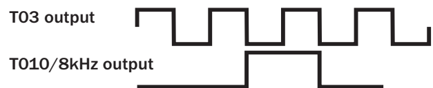
d) Pulse inverted, Reg.7A[3:2] = 11
