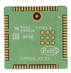
The SIM900 is a complete Quad-band GSM/GPRS solution in a SMT module which can be embedded in the customer applications.
