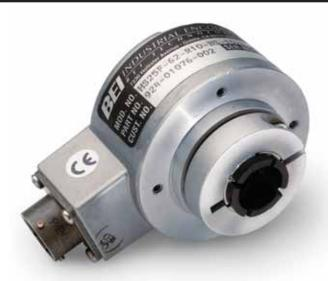
The HS25 combines the rugged, heavy-duty features usually associated with shafted encoders into a hollow-shaft style. Its design includes dual bearings and shaft seals for NEMA 4, 13 and IP65 environmental ratings, a rugged metal housing, and a cable gland.
