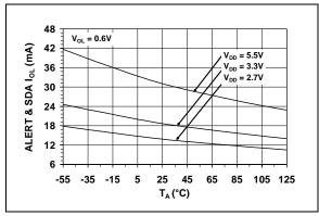
**FIGURE 2-7:** ALERT and SDA  $I_{\rm OL}$  vs. Ambient Temperature.
