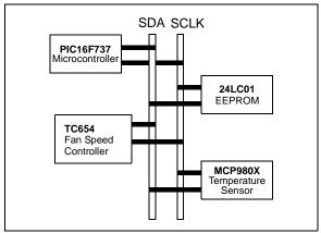
FIGURE 6-2: Multiple Devices on SMBus.
