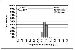
**FIGURE 2-4:** Temperature Accuracy Histogram,  $T_A = +25$ °C.
