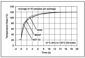
**FIGURE 2-9:** MCP980X Thermal Response vs Time.
