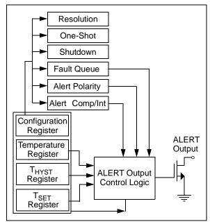
FIGURE 1: Register Block Diagram.
