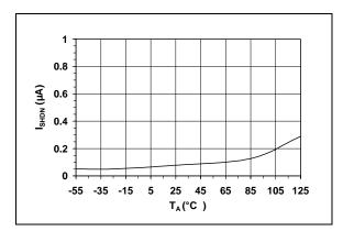
**FIGURE 2-6:** Shutdown Current vs. Ambient Temperature.
