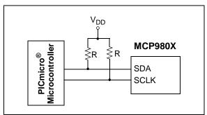
FIGURE 6-1: Pull-up Resistors On Serial Interface.
