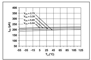
**FIGURE 2-5:** Supply Current vs. Ambient Temperature.
