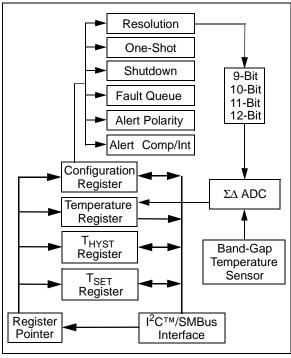
FIGURE 4-1: Functional Block Diagram.
