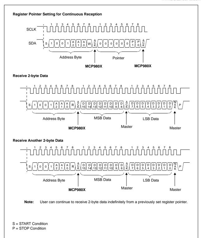
FIGURE 5-5: Receive 2-byte data from previously set pointer.
