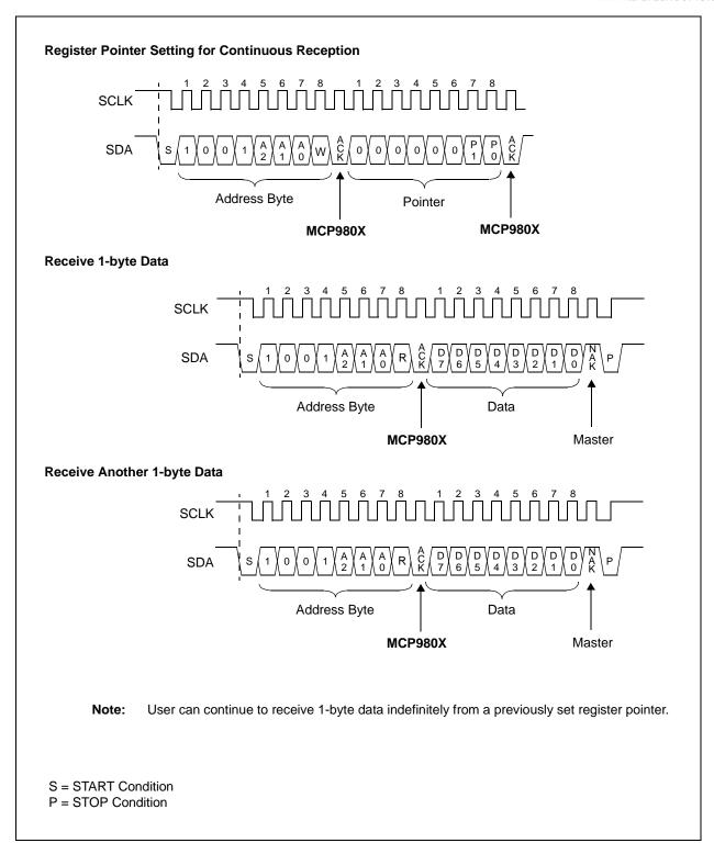
FIGURE 5-4: Receive 1-byte data from previously set pointer.
