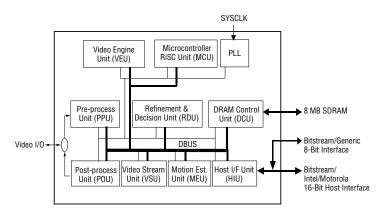
The CS92210 is a real time MPEG-2 video encoder and decoder (CODEC) that fully complies with the ISO/IEC-13818 Main Profile@Main Level (MP@ML) format, Simple Profile@ Main Level (SP@ML), and Main Profile@ Low Level (MP@LL).
