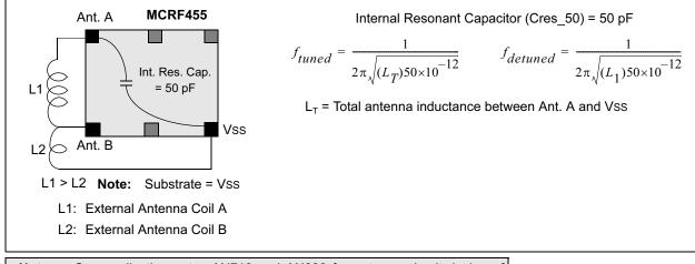
**Note:** See application notes AN710 and AN830 for antenna circuit design of Figure 2-2 through Figure 2-5.
