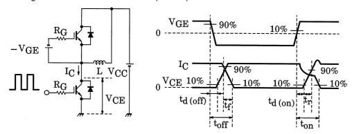
Switching loss measurement waveforms
