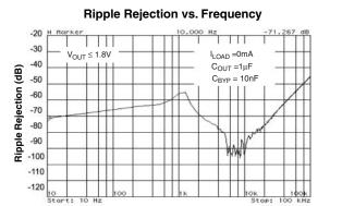
Ripple Rejection vs. Frequency
