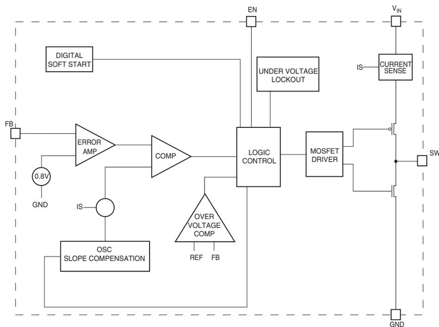
Figure 4. Block Diagram
