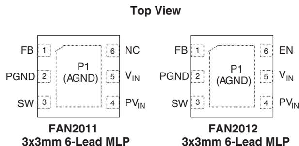
Figure 2. Pin Assignment
