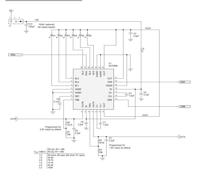
Figure 9: AAT2856 Section Schematic
