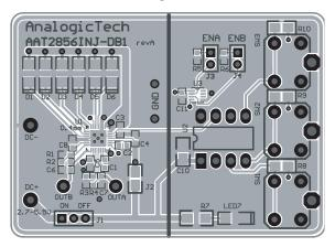
Figure 7: AAT2856 Evaluation Board Layout Top Side.
