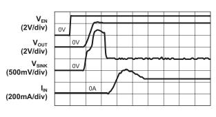
Turn On to 1.5X Mode Backlight (30mA/ch; Data 1; V<sub>IN</sub> = 3.4V)
