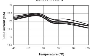
Turn On to 1X Mode Backlight (30mA/ch; Data 1; V<sub>IN</sub> = 4.2V)
