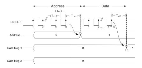
Figure 1: AS<sup>2</sup>Cwire Serial Interface Timing.
