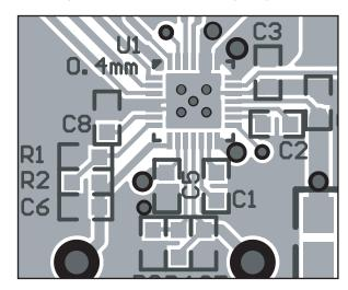
Figure 6: Example PCB Layout.
