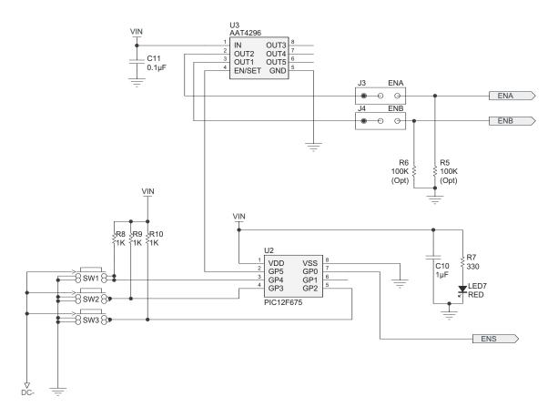
Figure 10: MCU and I/O Expander Section Schematic
