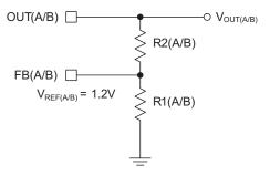
To select appropriate resistor values, first choose R1 such that the feedback network bias current is less than 10 $\mu$ A. Then, according to the desired V<sub>OUT</sub>, calculate R2 according to the equation below. An example calculation follows.
