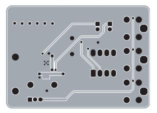
Figure 8: AAT2856 Evaluation Board Layout Bottom Side.
