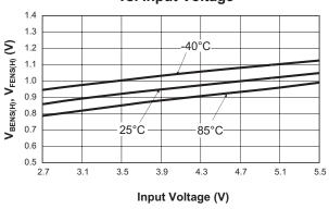
BENS, FENS Low Threshold Voltage vs. Input Voltage
