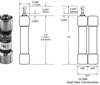
CATALOG SYMBOL: FNA (5AG) 1/10-10A DUAL-ELEMENT, TIME-DELAY 1/10 TO 30 AMPERES U.L. LISTED:
