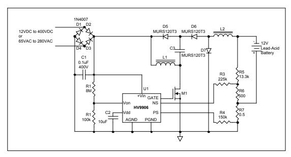
This floating battery charger circuit will charge a 6 cell 12V leadacid battery to a float voltage of 13.8V and provides a 1A charging current limit for a severely discharged or shorted battery. When the discharged battery terminal voltage is at 12V, the charging current is 130mA. The charging current decreases as the battery charges and the terminal voltage rises. When the maximum float voltage of 13.8V is reached the current into the battery will be essentially zero.
