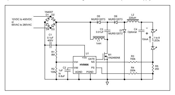
This circuit provides a constant average current output, which may be used to power LED lamps. The circuit maintains a constant average current and the value of C4 capacitor controls the peak-to-peak ripple, which decreases with increasing capacitor value.
