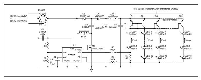
This circuit provides 0.5A constant average current output to power 249 LEDs , each operating at 20mA to form a large LED lamp or array. The circuit maintains a constant average current and the value of C4 capacitor controls the peak-to-peak ripple, which decreases with increasing capacitor value.
