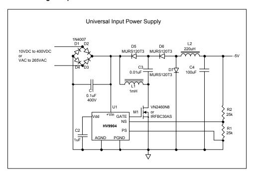
This circuit provides a non-isolated constant voltage output. The value of C4 capacitor controls the peak-to-peak ripple, which
