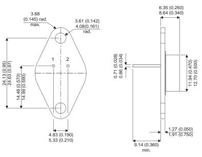
Bipolar NPN Device in a Hermetically sealed TO66 Metal Package.
