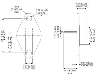
**Bipolar PNP Device in a** Hermetically sealed TO66 Metal Package.
