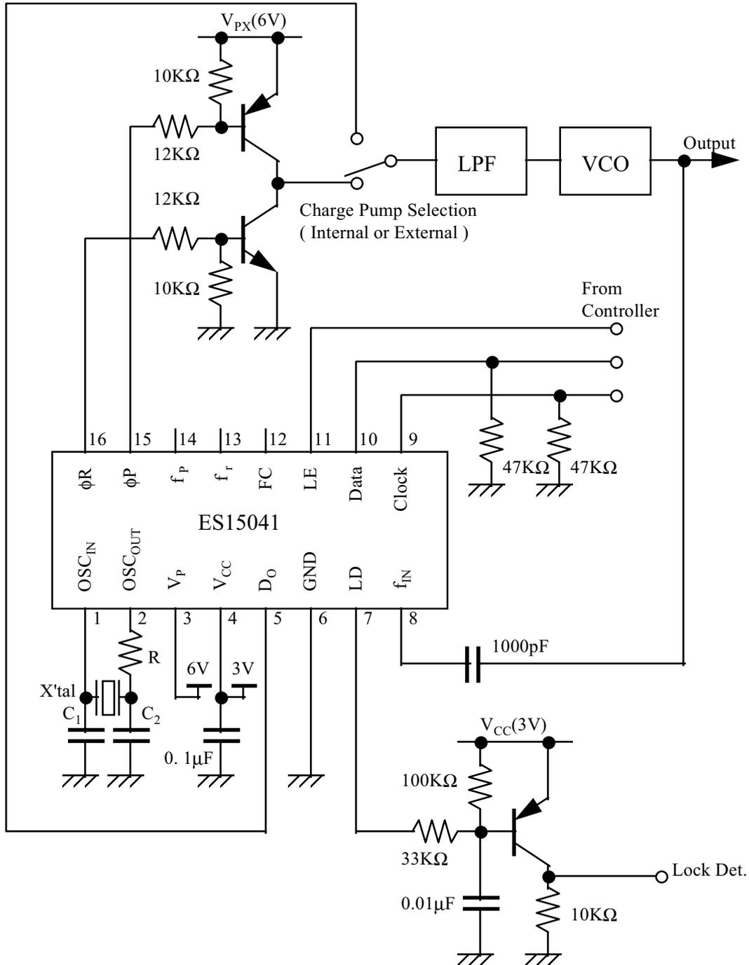
$C_1, C_2$  &  $R$  : Depends on crystal oscillator
