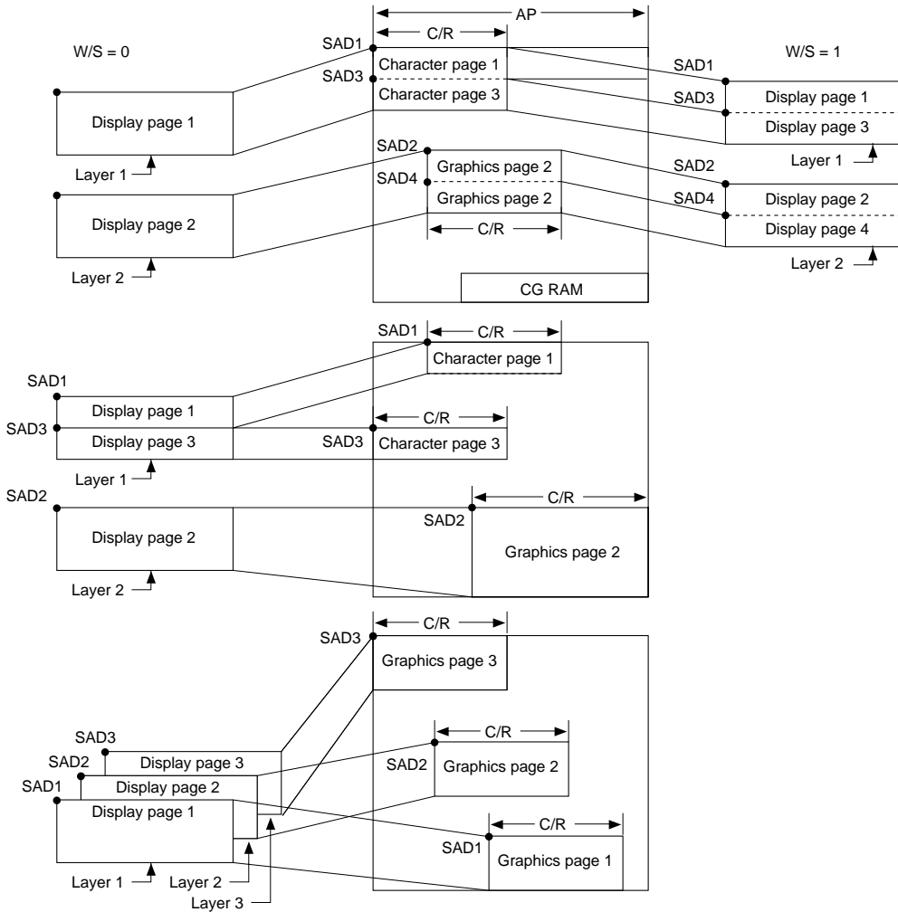
Figure 37. Display layers and memory
