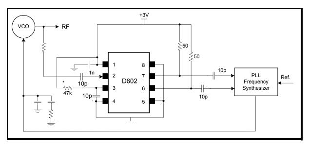
\* The 47k resistor provides a DC offset that disables self oscillation in the absence of an RF input.
