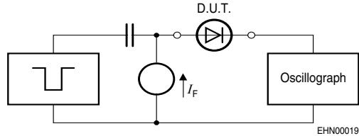
Pulse generator:  $t_p = 10\mu\text{s}$ ,  $D = 0.05$ ,  $t_r = 0.6\text{ns}$ ,
