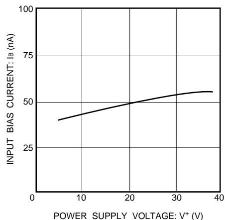
Fig.6 Input bias current vs. power supply voltage
