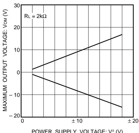
Fig.8 Maximum output voltage vs. power supply voltage
