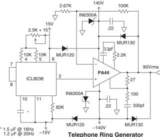
The PA44 is set for a gain of 38.5 boosting the 2.33V signal to 90V. The recommended compensation for gains above 30 is used. If capacitive loading is at least 330pF at all times, the recommended snubber network may be omitted. The 27 ohm resistor sets current limit to a nominal value of 111mA to insure peak currents out of at least 78mA.
