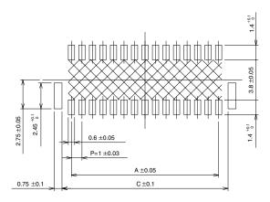
Note: Shaded area must be free of any electrically conductive traces to avoid contact with soldered pin header terminations.
