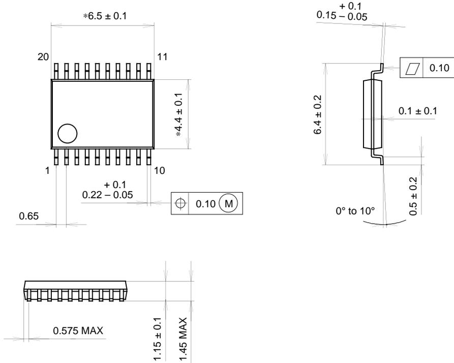
NOTE: Dimension "\*" does not include mold protrusion.
