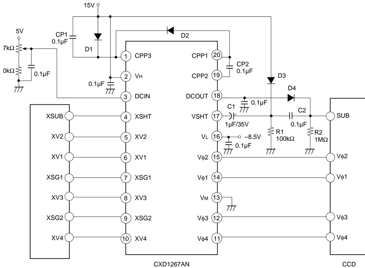
\* A peripheral circuit can be simplified by CCD image sensor.
