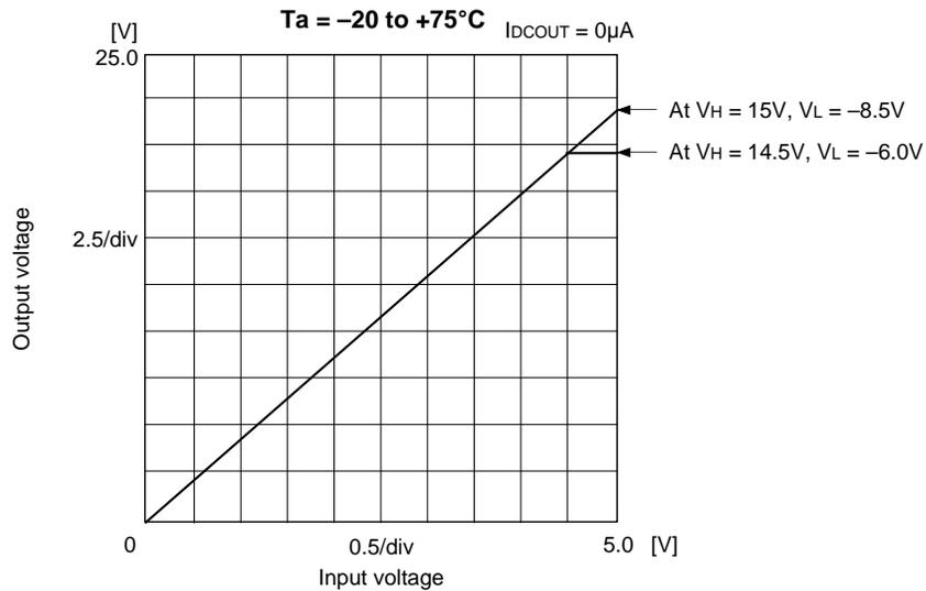
**Note)** Operating amplifier maximum output voltage is restricted as shown in the formula below depending on supply voltage setting of  $V_H$  and  $V_L$ .
