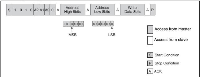
Note: In the MB85RC64, input "000" as the upper 3 bits of the MSB.
