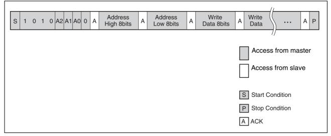
Note : It is not necessary to take a period for internal write programming cycles from the buffer to the memory after the stop condition is generated.
