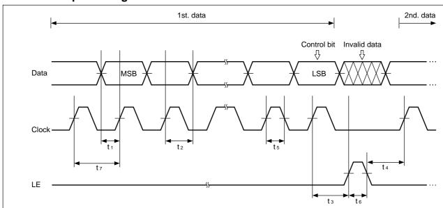
On rising edge of the clock, one bit of the data is transferred into the shift register.
