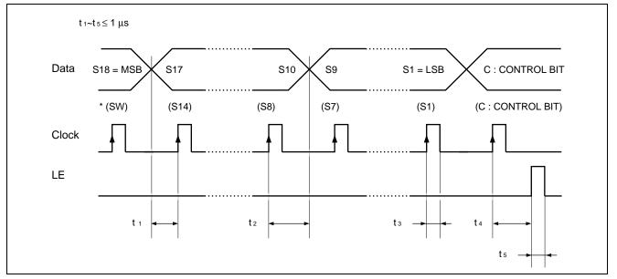
Notes: Paranthesis data is used for setting divide ratio of programmable reference divider. On rising edge of clock shifts one bit of data in the shift register.
