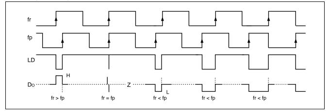
Phase comparator output waveforms are shown below.
