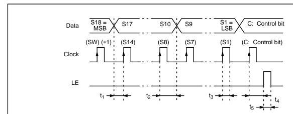
\*1: Bits enclosed in parentheses are used when the divide ratio of the programmable reference divider is selected.
